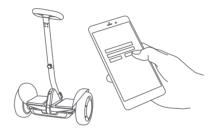
3 Click Device > Search Vehicle to connect to your S-Max. The S-Max will beep when the connection is successful. The Bluetooth icon will stop blinking and remain illuminated.
