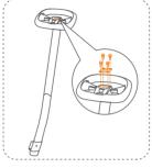
Open the battery cover of the control panel. Place in two AAA batteries. Snap the cover.
