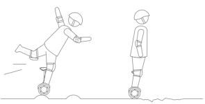
When traversing small bumps or uneven terrain, maintain a moderate speed of 2–6 mph (3–10 km/h) and keep your knees bent. Do not go too slow or too fast; otherwise, you may lose control and fall.
