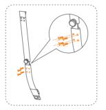
Align the flange with the holes on the steering wheel and tighten it with four M5 screws with the 4 mm hex wrench.
