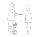
2 Lightly place one foot on the foot mat, while keeping your other foot on the ground holding your weight. Do not press the steering bar with your leg.
