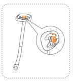
6 Insert the LeanSteer into the vehicle body and tighten the two M5 screws with the 4 mm hex wrench.
