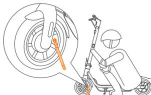
1 EN Unscrew the valve cap.
