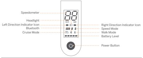
Power Button: Press the button to power on; press and hold the button for 3 seconds to power off. When the KickScooter is on, press the button to turn on/off the headlight and the tail light, and press twice to switch between the speed modes.
