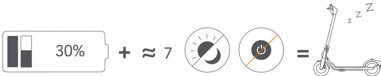
EN When the scooter is not powered on for about 7 consecutive days and its battery level is less than 30%, the battery will enter into sleep mode. If this happens, your scooter cannot be powered on. Please charge the scooter.
