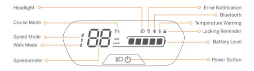
Power Button: Press the button to power on the scooter; press and hold the button for 3 seconds to power it off. When the scooter is on, press the button to turn on/off the headlight and the tail light, and press twice to switch between the speed modes.
