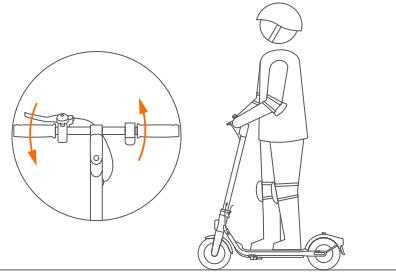
④ EN Slow down by releasing the throttle and squeezing the brake lever. **The rear light flashes when braking.**
