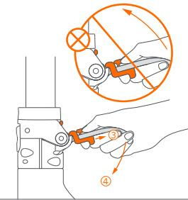
**1** **EN** Lift the safety lock and open the quick-release lever.
