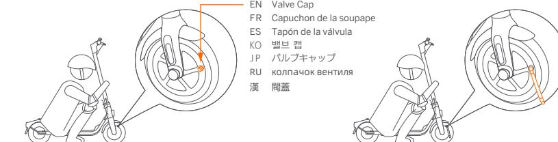
1 EN Unscrew the valve cap.
