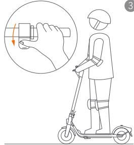
③ EN Put both feet on the footboard and stand stably. Press the throttle to speed up when you are balanced. **Note: For your safety, the motor will not engage until the KickScooter reaches 1.9 mph (3 km/h).**
