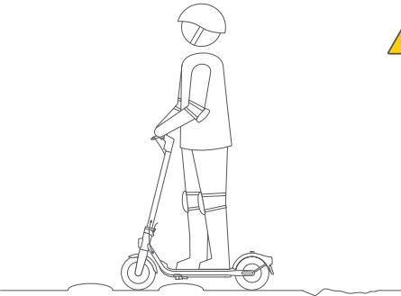
EN Keep your speed between 3.1–6.2 mph (5–10 km/h) when you ride through speed bumps, or other uneven surfaces.
