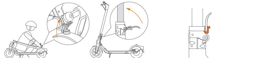
1 EN Disengage the snap hook from the buckle.
