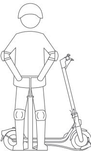
3 EN Connect the pump to inflate the tire.
